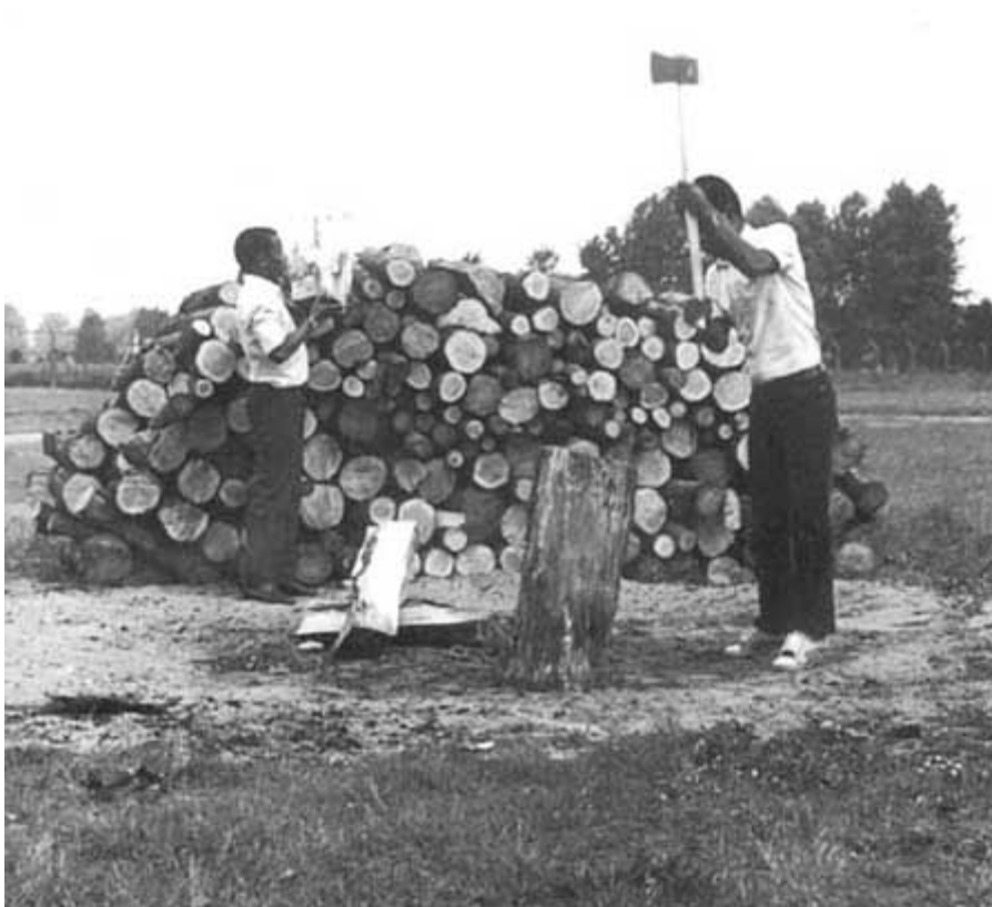
Photo. 27. Wood preparation for charcoal. Note short length of wood. Photo TPI
