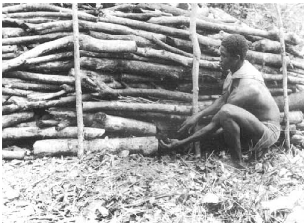
Photo. 10. Earth mound kiln under construction showing firing point. Ghana. Photo Lejeune.
