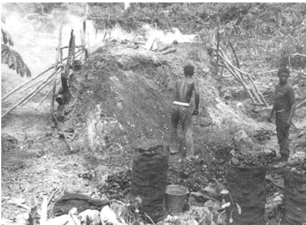
Photo. 12. Unloading charcoal with sacks from earth mound kiln. Note rake used to separate soluble charcoal from earth covering in early stages of unloading. Ghana. Photo Lejeune.
