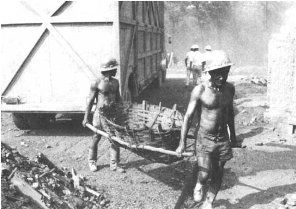
Photo. 38. Basket used to unload charcoal from brick kilns. Note high side charcoal transport truck. Minas Gerais, Brazil. Photo. J. Bim
