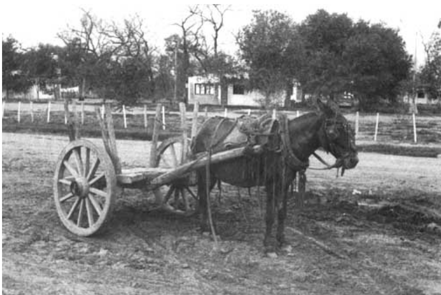
Photo. 2. Mule cart or "zorra" to transport wood billets from stumps to round side and sometimes to kiln where distances are short. Salte, Argentine. Photo J. Bim.
