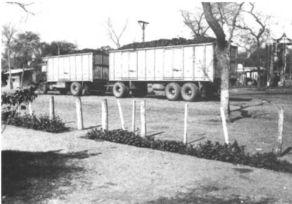
Photo. 37. High side truck and trailer for charcoal transport. Note position of unloading doors in sides. Salta, Argentina, Photo. J. Bim
