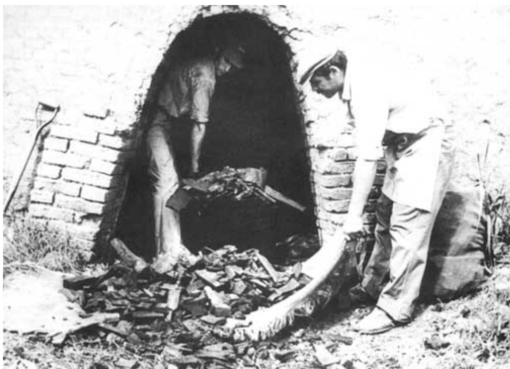
Photo. 24. Unloading charcoal from a brick kiln in Salta, Argentina. Fork is used to allow fires to be separated. Photo M. Trossero
