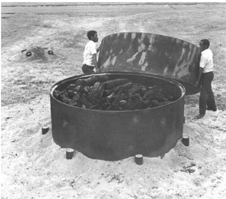
Photo. 35. During carbonization period wood has been reduced to about half its original volume. Photo. TPI
