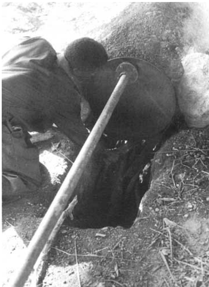
Photo. 25. Retort made from oil drums. Note pipe to collect condensate and fire laid in trench. Ghana. Photo Lejeune.
