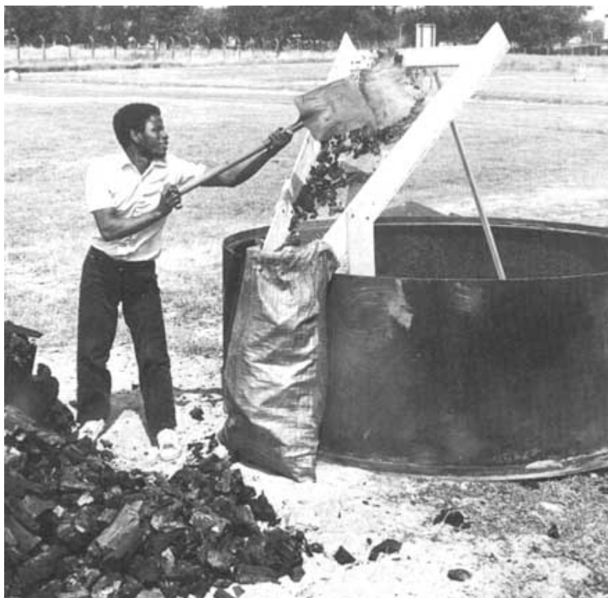
Photo. 36. Sieve chute should be used to separate the large charcoal pieces from fines and dust. Photo. TPI
