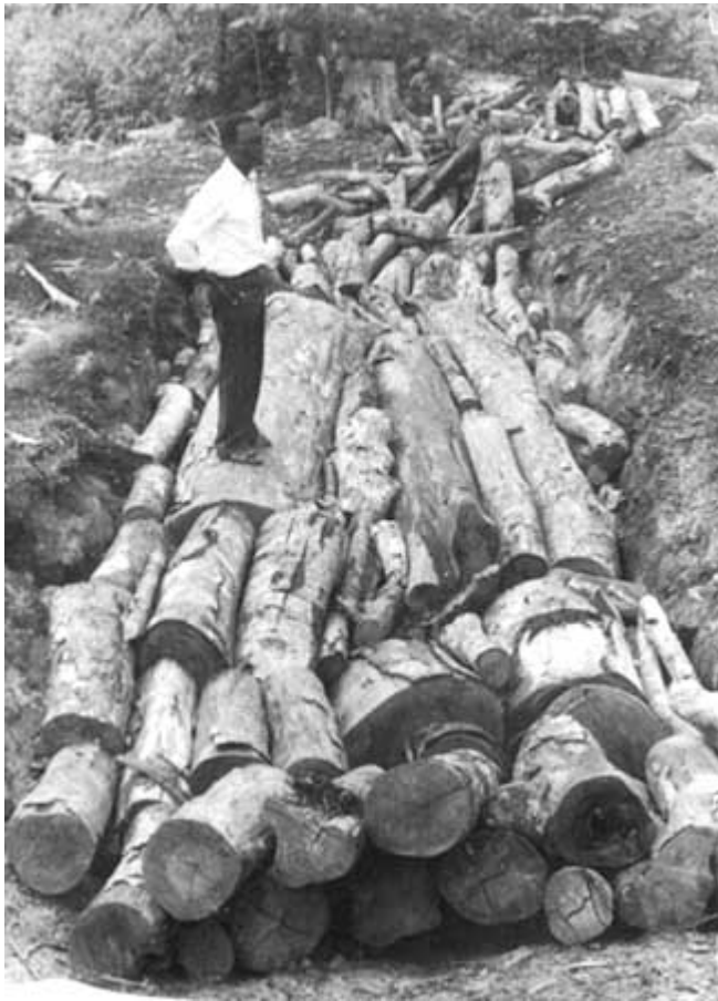
Photo 6. Earth pit kiln during loading phase. Note large diameter round timber which can be used. Ghana. Photo Lejeune.
